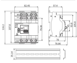
Note: Terminal wiring area: fit for (1~25)mm<sup>2</sup>.
